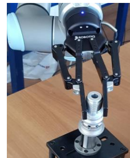
Figure 4. UR10 manipulator robot with 2F-140 adaptive gripper
